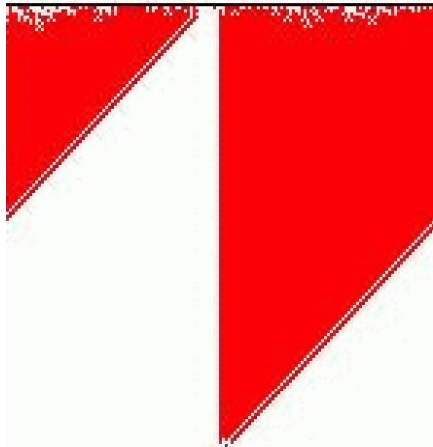
Figure 2: Space-time diagram of block expansion rule \phi_{\text{block}} when applied to the density task.
