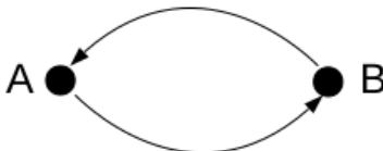
Figure 8: The catalysis graph of the simple 2-reaction RAF set in Figure 5. The two molecule types A and B mutually catalyze each other’s formation, creating a closed loop in the catalysis graph.
